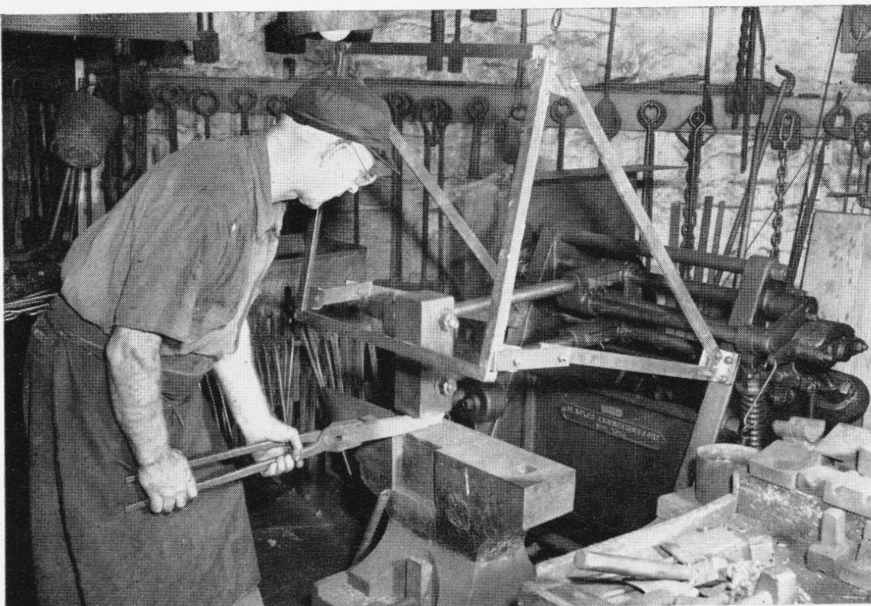
Fire spewing from a smithy's forge and white-hot metal particles flying from work under the blows of a heavy hammer have always been part of the color and atmosphere of a blacksmith shop. The color and atmosphere are still there, but not the danger from flying particles. This power-driven sledge hammer and anvil covered with a non-shatterable glass pane protects the smithy from chips of hot metal that fly under the hammer's impact.
