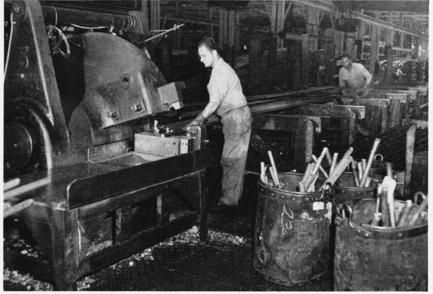
Testing for casting defects in brass rods, Sam Behuniak cuts off a rod end on the alligator shears while Robert Johnson feeds the rods forward. The rod ends will later be tested and separated according to their alloy before being sent back to the Casting Shop for recasting. The barrels at right contain different alloys of brass.
